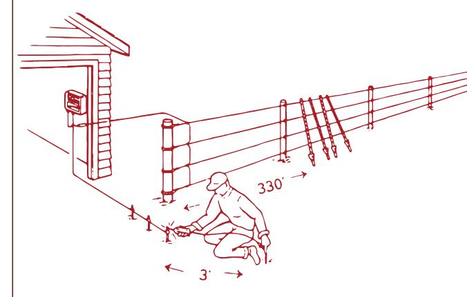
**STEP 1.** Create a dead short on the fence line, preferably 330 ft. from the ground rods, or as far as possible if the fence is less than 330 ft. Lean steel posts on a hot wire as shown.
