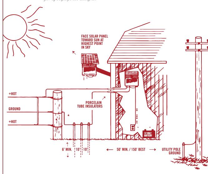
\* A return ground system as show may not be necessary if adequate moisture and soil conductivity are present.
