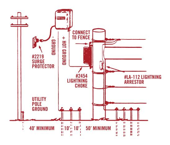
In severe lightning areas, installing a Lightning Arrestor with ground rods every 1/4 mile of fence line is recommended.
